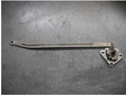
1964-66 interior handle regulator strap connects here.
