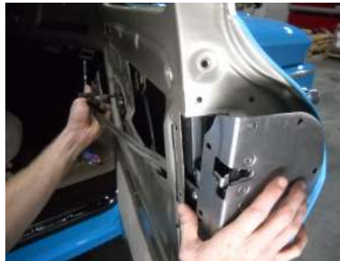
1964-66 interior handle regulator strap connects here.
