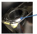
Depending on your tailgate the delrin (black piece) with Beveled edge could be installed inside the cup pocket or like it is shown – Ensure it's Installed flush or just below flush of the tailgate edges.
