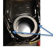
Flat edges on each side, installed where it fit best, prevents it from spinning
