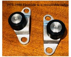
Pre-check to ensure proper installation. Test fit the female delrin bearing on both sides. If it goes in tight it will be very difficult to install the trunnion bracket (stainless) ball and will be tight while opening and closing the tailgate. You could sand the edges of the Delrin bearing (black parts) to make it fit better, tight but not to tight. Go slow and it just might need to be sanded a little more, the key it that you don't want the delrin (black part) to spin at all. Continue to check
