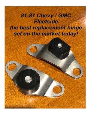
They should install like the originally installed, they were made from the reproduction models on the market today. Check to ensure proper installation. By test fitting the female delrin bearing on both sides. If it goes in tight it will be very difficult to remove the tailgate. You could sand the edges of the Delrin bearing (black parts) to make it fit better, tight but not too tight but not too loose.
