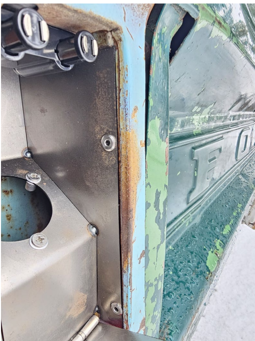
Photo 3: Bucket seated in taillight opening.
