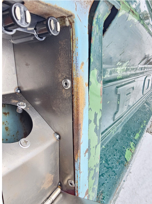
Fuel filler bucket installed behind the taillight opening.
