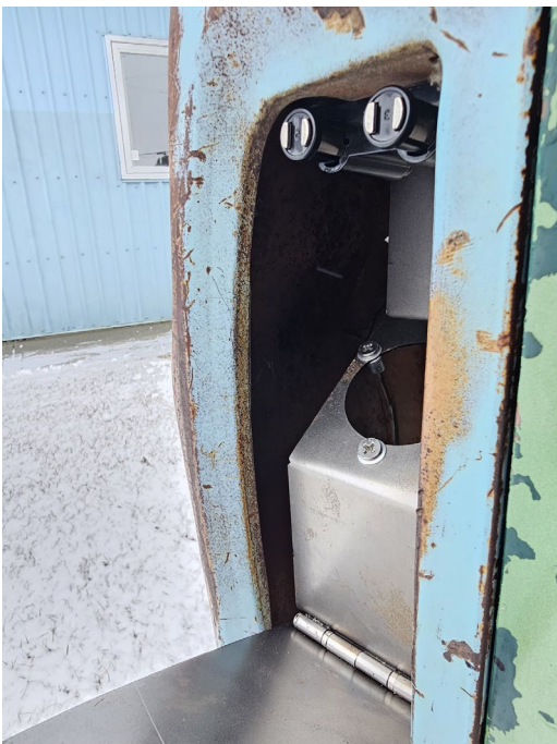
Photo 1: Taillight opened to access fuel cap.
